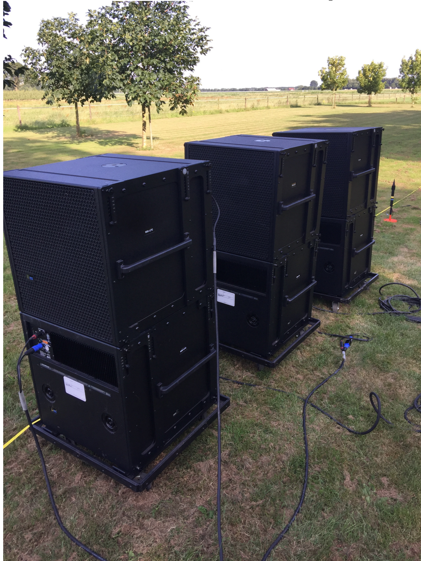
End Fired Array 3 x Front/Back stack (TBG (= Timo Beckman Geluidstechniek))
